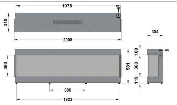
FRAME BUILD OUT DIMENSIONS (All dimensions are in millimetres)
