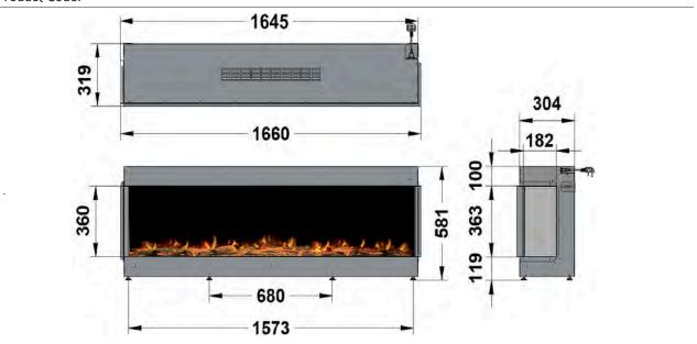
FRAME BUILD OUT DIMENSIONS (All dimensions are in millimetres)
