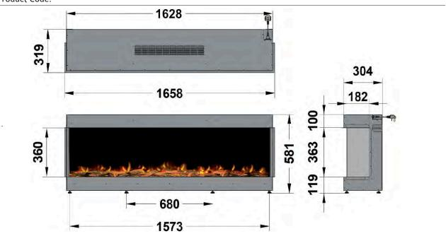
FRAME BUILD OUT DIMENSIONS (All dimensions are in millimetres)
